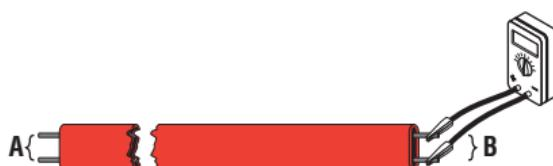
The approximate location of the fault, expressed as a percentage of the heating cable length from the front end (A) is:
